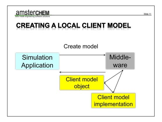
To create a client model, the simulation application can ask the middle-ware to do so, and the middle-ware returns an object representing the client model. This object will internally communicate with the client model implementation and with the middle-ware (for example to allocate data structures). In effect, the simulation application talks directly to the client model implementation. This is in the case the client model is implemented locally based upon the new middle-ware.
