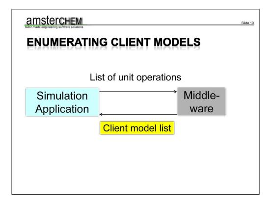
To start, the simulation application asks the middle-ware for a list of installed client models of a particular type, for example unit operations. The middle-ware returns an enumeration class with all locally and remotely registered unit operations, including COM based ones. The simulation application can have the user pick an entry from the list, based upon name and description, and instantiate it.
