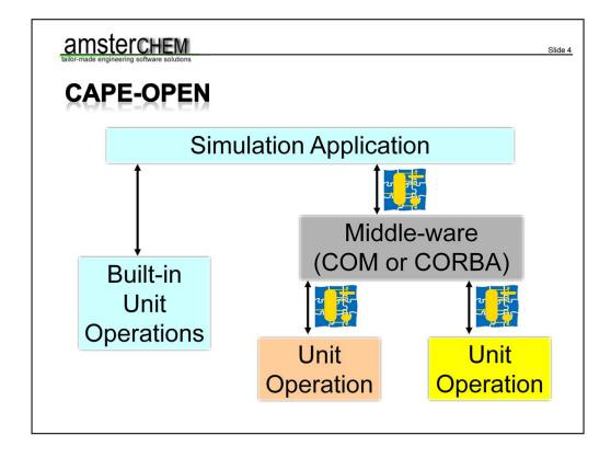
For flowsheeting applications, another class of models used is Unit Operations, that represent physical equipment, such as a pump, a reactor, a separation tower.... The same story holds; a simulation application will likely have built-in Unit Operation models, and likely provides some custom way of interfacing with user models. If in addition a CAPE-OPEN Unit Operation plug is implemented by the simulation environment, third party or user unit operations that expose a CAPE-OPEN plug can be used.
