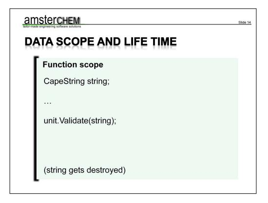
The data scope should be fully automatic. The coder should merely create an object of the proper data type. As an example, this slide depicts the scope of a function. Inside the function, a CapeString variable is declared. This string variable is passed to a CAPE-OPEN function, here for example Validate of an ICapeUnit interface. At the end of the function, the string variable automatically goes out of scope, which takes care of releasing the memory associated with the string data.
