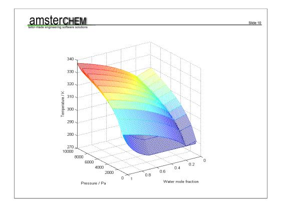
... we see here a phase envelope for the Water / n-Butanol system at various composition and temperature. Such a plot allows us to inspect the shape of the phase envelope within the region of interest for a quick analysis of what our process model may do under certain conditions. The code to generate the data is shown on the next slide.
