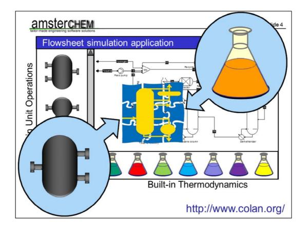
Fortunately such a universal interface exists. It is called CAPE-OPEN. It is an industrial, freely available, open software standard that allows exchange of chemical engineering software components, particularly unit operation models and thermodynamic models, between simulation applications. It is maintained by the CAPE-OPEN organization CO-LaN, and available from their web site.
