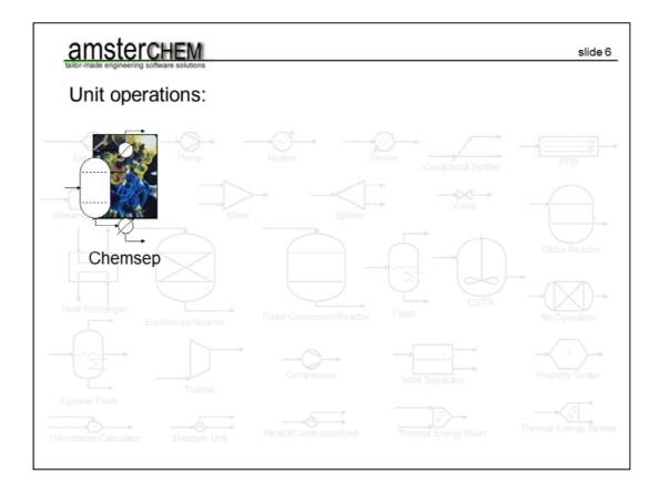
the Chemsep unit operation for distillation and extraction columns. The authors of Chemsep contributed immensely to the development of COCO, and the thermodynamics are still largely based on their code and data. The ChemSep unit operation is the main seperation device in COCO.
