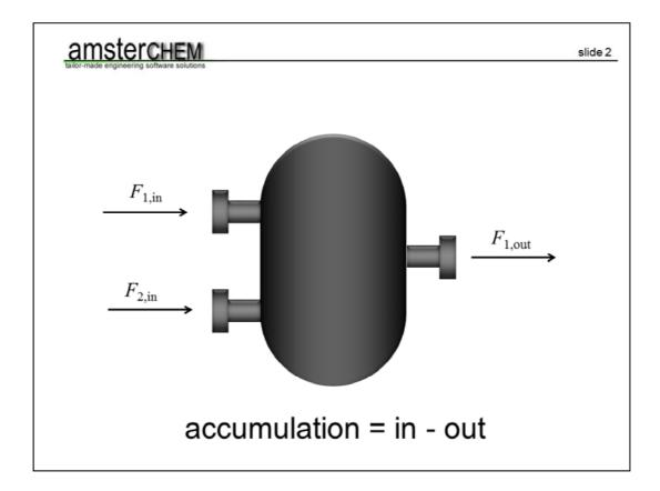
We can break the factory down into smaller pieces. Such a piece is called a unit operation. Also around a unit operation, mass and energy are conserved. The accumulation of mass and energy in the equipment equals what goes in minus what comes out.
