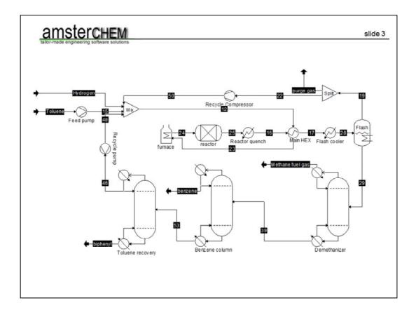
For a single unit operation, the mass and energy balances may be easy to solve. However, in a real process we typically deal with recycles. This is where flowsheet modelling comes in. A flowsheet model gives us a mathematical description of the factory. We can use the mathematical model to design and optimize the process, to do if-then studies and to come to a better overall understanding of the factory.
