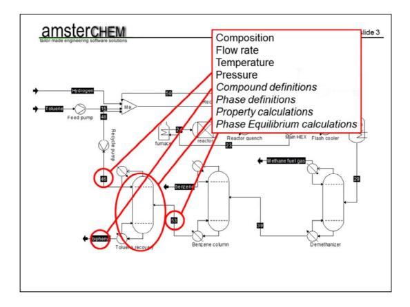
And remember that it is the unit operation that actually performs the local balance. So it too must have access to the thermodynamic property calculations
