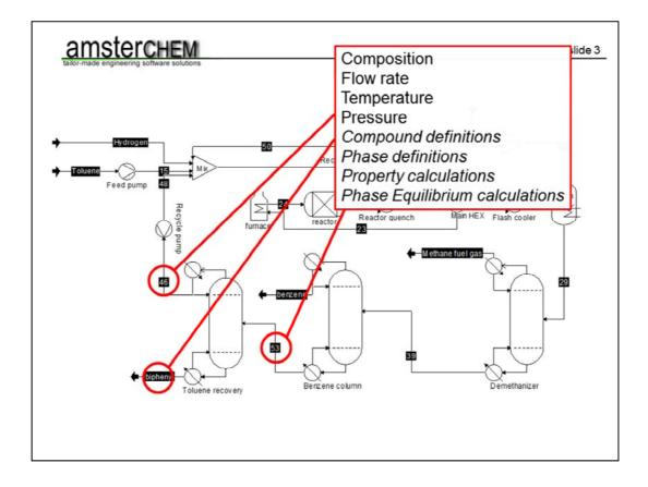
It stands to reason that if we are interested in closing energy balances, that the definition of thermodynamics must be consistent on the streams that go into and come out of a given model. Otherwise we are comparing apples and pears in the enthalpy balance.
