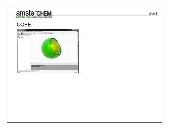
COCO is a bit different from other simulation environments. It is assuming from the start that you want to mix and match. We have as the basis, COFE, the CAPE-OPEN Flowsheet Environment. COFE does not feature any built-in unit operation models or thermodynamics. It does not make any assumptions on the type of unit operations, number of compounds, maximum number or types of phases or anything else, as this is defined by external software components.
