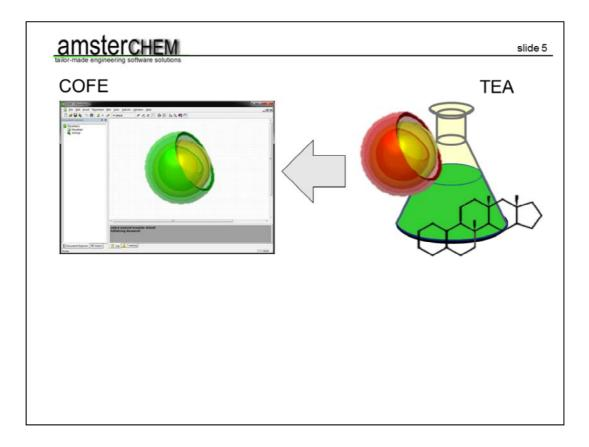
The thermodynamics that come with COCO are provided by TEA, Thermodynamics for Engineering Applications. TEA includes more than 100 property calculation methods. The default data bank contains over 400 compounds, and can easily be extended.
