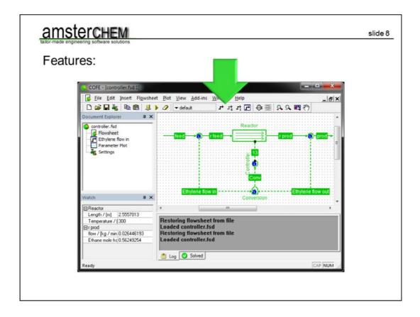
intuitive toolbar buttons for inserting objects like streams and unit operations,
