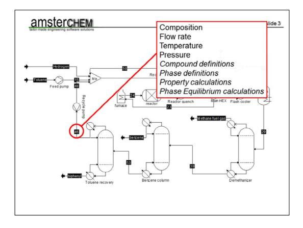
Clearly, any material stream is represented not only by a flow rate, but also by a composition, and additional conditions like temperature and pressure. In addition to the conditions, there is an underlying definition of the thermodynamics. This includes chemical compound and phase definitions, but also a selection of models that allows for the prediction of physical and thermodynamic properties and phase equilibria.
