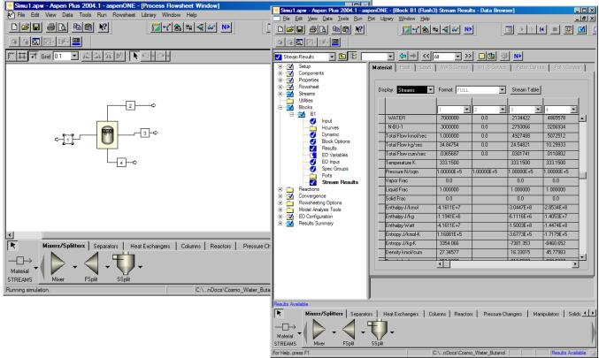
Figure 5: AspenTech's AspenPlus 2004.1 three phase flash using TEA thermodynamics combined with COSMO*Logic*'s activity calculation routine COSMO*Therm*, as presented by Frank Eckert at the annual CAPE-OPEN conference in Cannes (France), March 2006.
