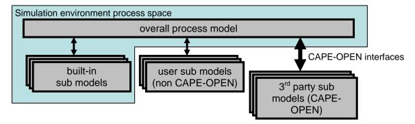
Figure 1: typical setup for process engineering modeling tools supporting CAPE-OPEN models.
