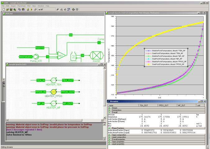
Figure 3: screenshot of COCO showing two open flowsheet documents. The document on top shows comparison of thermodynamic calculations of three different vendors. The stream view on the bottom right lists the results of the stream exiting the heaters (with equal configuration and equally defined inlet streams). The plot on the top right shows the phase envelopes for the three thermo systems at inlet stream conditions.
