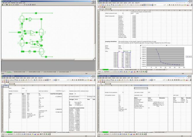
Figure 4: COFE flowsheet in Microsoft Excel. A) The flowsheet document embedded in Excel. B) Thermodynamic calculations utilizing the flowsheet's thermodynamic setup C) accessing stream data from the flowsheet D) accessing unit operation data from the flowsheet.
