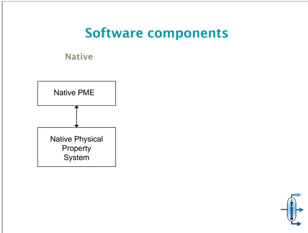
This diagram shows the typical configuration of a Process Modelling Environment (PME) with its own physical property system. Typically the interface between the two will be proprietary and designed to match the way that the PME works. It should be efficient because the PME and property system 'know' each other. Links can be direct and in some older systems the two components would be tightly integrated.
